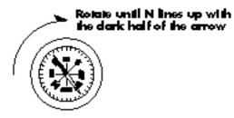
3. Locate the tick mark on the compass edge that corresponds to the **azimuth** number you wrote down. This is the direction of your azimuth setting (the direction the dish will need to be pointed to receive signals from the satellites). Pick a landmark or lay down a stick in that direction for reference from the mounting location.
